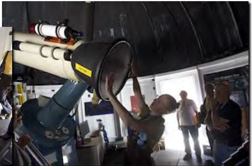
Left: At the observatory in front of the Air and Space Museum, John Dobson's Solar Telescope is displayed for us. Right: Shauna Edson describes a HUGE Sun Gun attached at the end of a 4" refractor. PVC helps attach the gun, made of a decent sized planter with screen material designed for rear projection as the observation area. A really large display is created.
