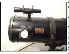
accessories include a 6x30mm finder and three eyepieces with focal lengths of 9mm, 12.3mm and 40mm. SLAS plans to add this to the Loaner Scope Program in the near future.
